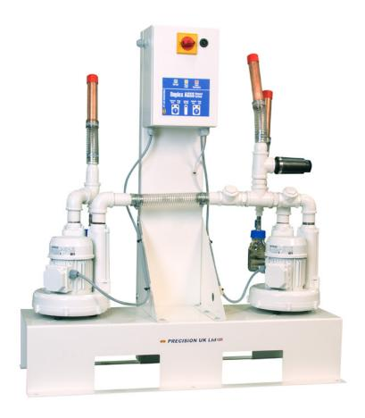
Precision UK's CPX AGSS Plant is manufactured under BS EN 13485 Medical Devices: Quality Management Systems. It provides a centralised or dedicated source for the safe removal of exhaled anaesthetic gases from within the theatre, available in simplex and duplex pump configurations dependant on individual requirement.
