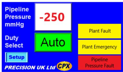
a. Yellow Plant Fault :- illuminate's in the event of any single fault
